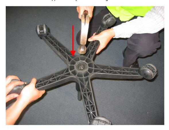
2. Using a hammer, hit the centre of the base
